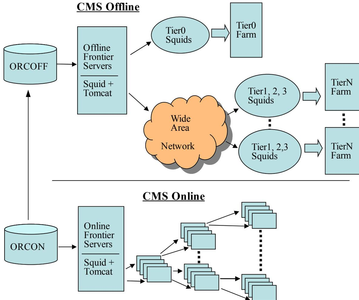
**Figure 1.** How Frontier is used in CMS
